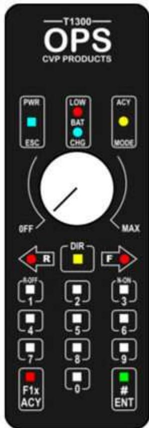
**What is a DCC Throttle used for?** This is a very important part of operating the layout. It is the connection between you and the way the train runs, this applies to any DCC layout. On the GNDU I use the **EasyDCC Throttles by CVP**. As its name implies it is a throttle not a walk around command station as used on some systems – it is purely for driving the train with no programming involved.
